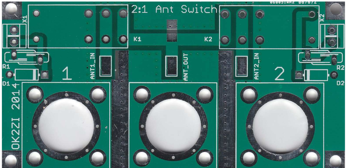
Bare PCB, the size is 49x100 mm
