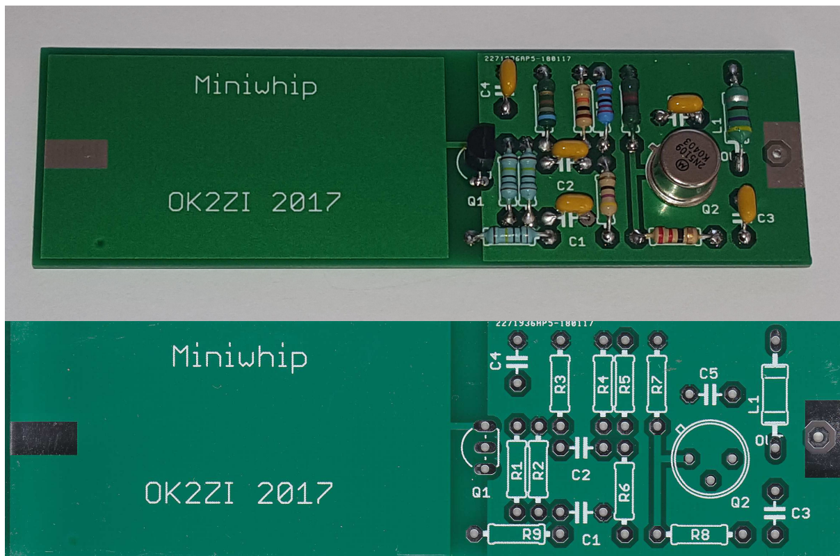
Antenna schematic and finished PCB
